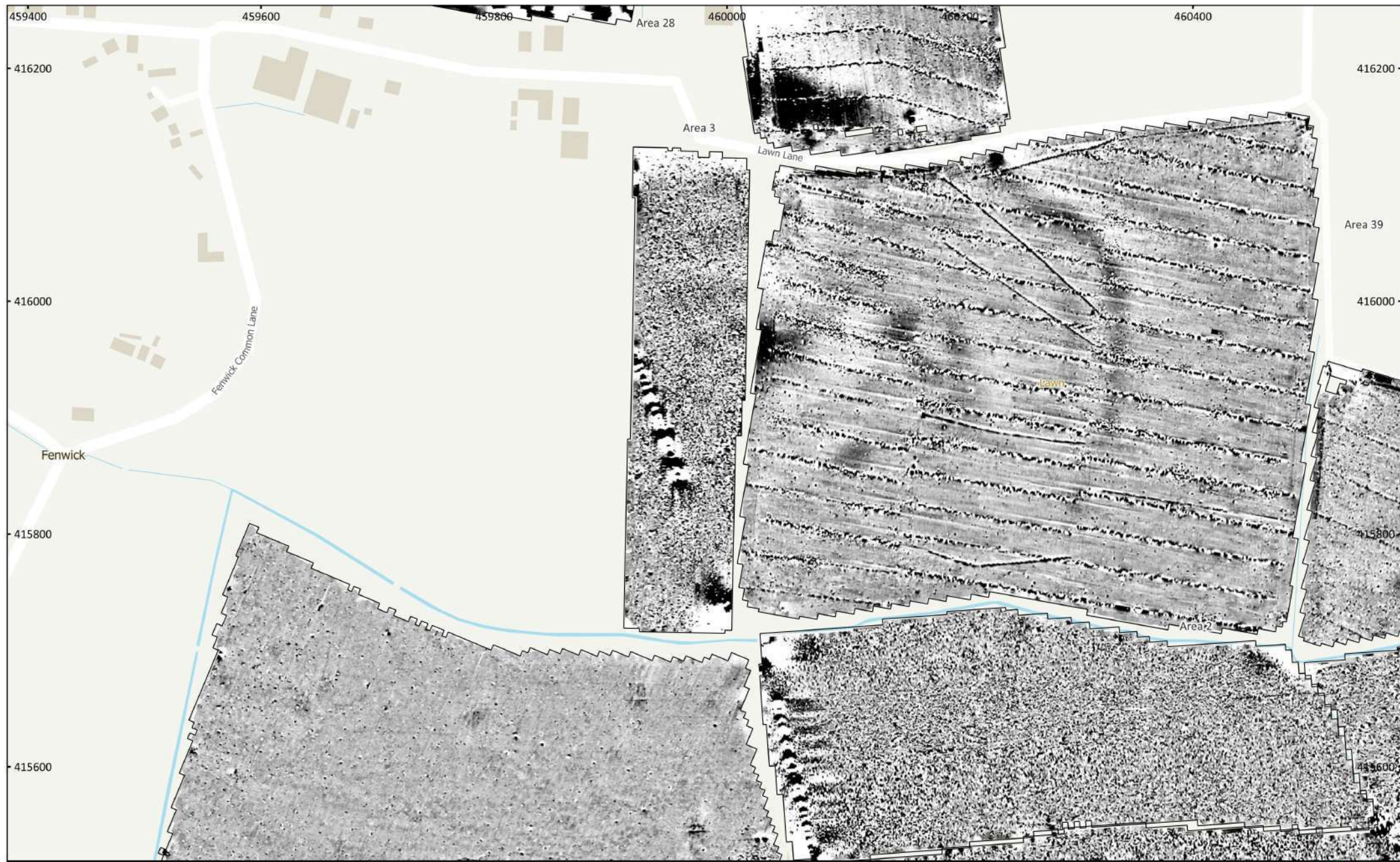
MSSE1569 - Fenwick Solar Farm Scheme, Doncaster Figure 21 - Magnetic Total Field (Lower Sensor) (West) 1:3,000 @ A3 Copyright Magnitude Surveys Ltd 2023 Contains Ordnance Survey data © Crown Copyright and database right 2023
